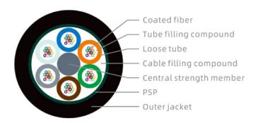
The GYTS cable is to sheath 250µm fiber into PBT loose tube with water-resistant jelly filled. All the PBT tubes (and fillers) are stranded around the central strength member and covered by plastic coated steel tape (PSP) into a compact and round shape. Between the fibers and tubes, the water blocking compound is filled for water resistance. Finally, the cable is completed with a PE sheath.
